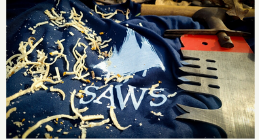
Saw noodles created after testing a freshly sharpened crosscut saw placed on top of a SAWS uniform.
